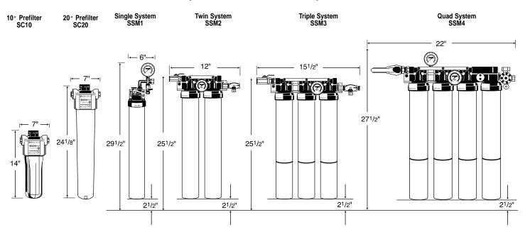
IMPORTANT: Must have minimum 21/2" clearance for cartridge change.
